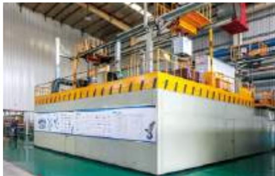
水平连铸炉 Horizontal continuous casting furnace
