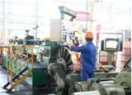
复绕机 Rewinding machine
